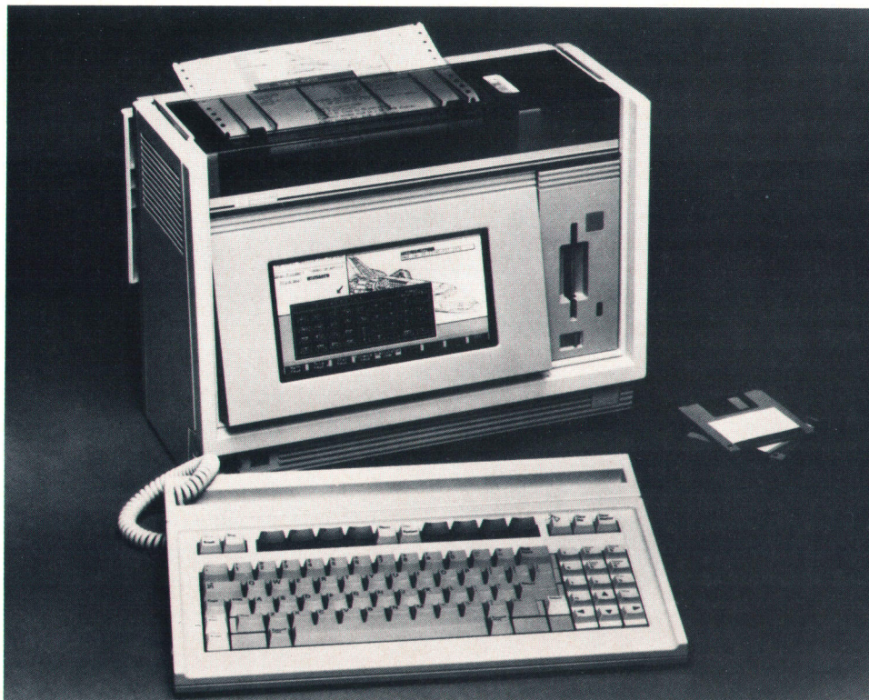
Fig. 1. HP's Integral Personal Computer is a powerful multitasking computer system in a 25-lb transportable package. Designed for technical professionals, it features a built-in ThinkJet printer, a double-sided, double-density 3½-inch disc drive, a 255×512-pixel, bit-mapped electroluminescent display, and an HP-IB interface.
